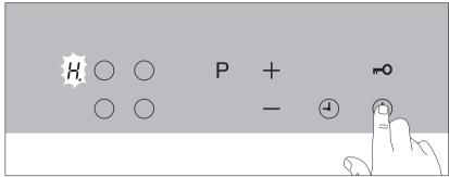
When an individual cooking zone or the entire hob is switched off, any residual heat is shown with an [H] (for "Hot") in the digital display for the appropriate cooking zones.
